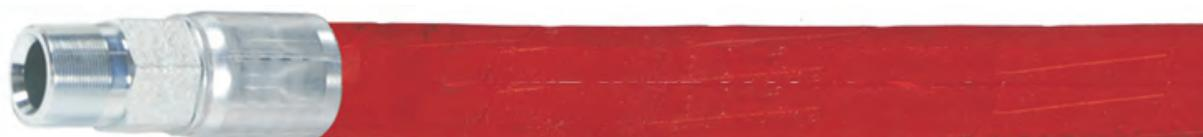
BOP hose range is designed for emergency situations where operation must continue in fire conditions. BOP hoses are wholly bonded rubber construction with embedded fire resistant properties offering relatively light weight and maximum flexibility. There is no need for additional materials to be added around the hose to achieve the fire resistance. BOP hose is clearly recognisable with the outer red cover.
