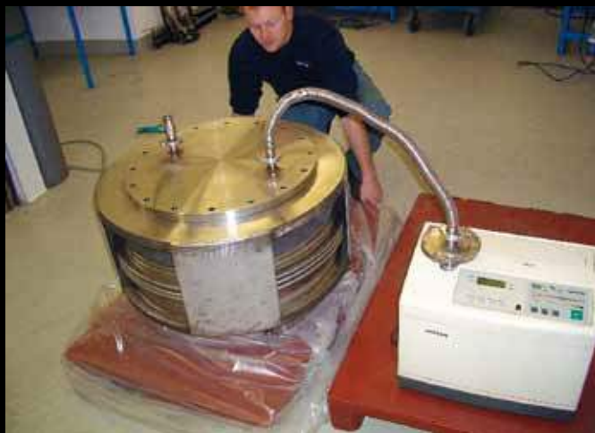
Helium leak test
