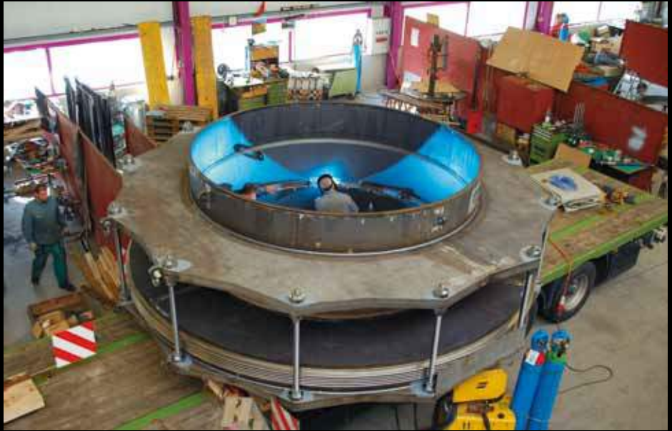
DN5000 pressure balanced expansion joint manufactured and delivered on customer's site in less than 4 weeks
