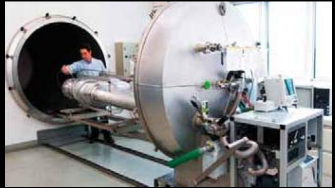
Integral test in vacuum chamber
