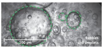
The properties of droplets in multiphase systems (e.g., water/oil) influence separation efficiency and mass transport. Knowing their size will enable you to minimize energy cost and waste.
