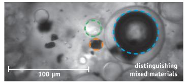
Real processes and materials vary in their properties and nature. Our intelligent software is able to distinguish between different materials and render separate size and characteristic distributions accordingly.
