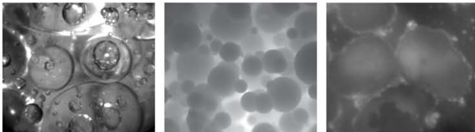
< Styrene droplets in water at the beginning of polymerization, Polystyrene resin particles in a fluidized bed, Polyvinyl chloride particles from a pilot plant after reaction in a stirred-tank.
