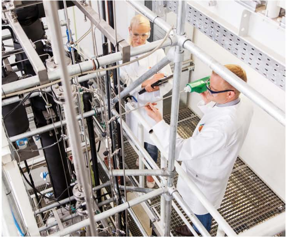
Installation of the SOPAT-VR for the determination of the size of dodecene droplets in H 2 O from a mini-plant. >
