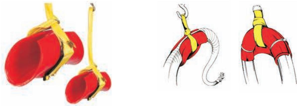
A PUHB Hose Saddles is a polyurethane saddle designed to suspend hoses. Each model comes complete with its own UV treated polyester sling which is fastened in a choker position. The PUHB Hose Saddle is designed to accommodate the manufacturers' minimum bending radius to protect hose from kinking and prolong the life of the hose.
